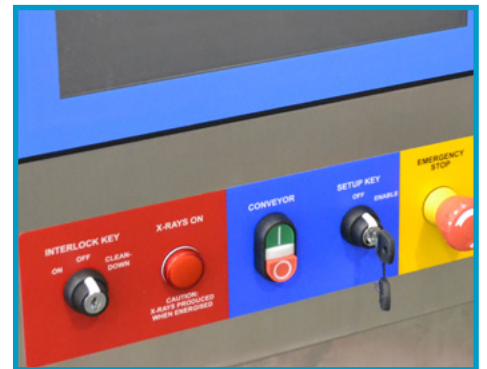
Critical controls are placed within operators reach
